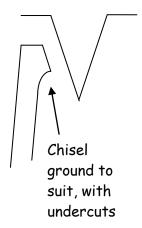
Now turn out the recess for each point of the star. Each recess will eventually have a temporary cap fitted to it, with a small recess in, the idea being to support each star point when you're doing the next one. Each cap will be 26mm diameter.
