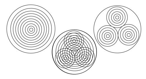
The object of the demonstration was to produce in a 6mm thick disc, a series of concentric rings 3mm thick, 3mm deep on one side, then on the other side to produce three sets of concentric rings with centres differently placed from the original rings, also 3mm deep, such that the rings would break through into one another so that in places you could see from one side through to the other.
